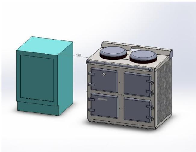
Minimum 450mm on left hand side of cooker to nearest cupboard or flammable material.
