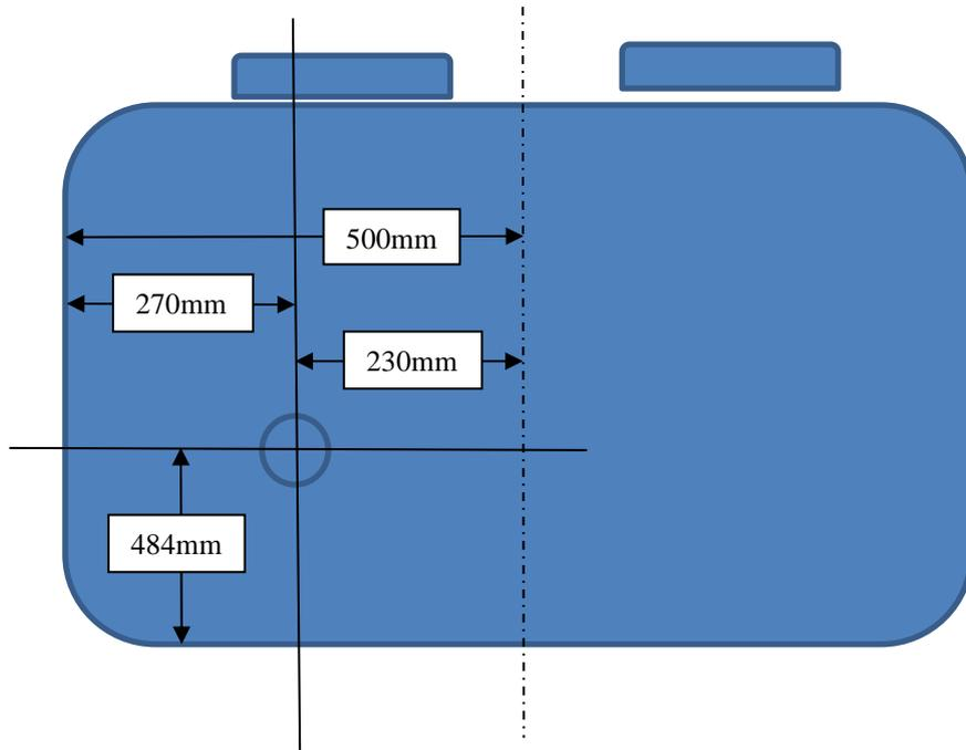
This diagram shows the position of the air inlet on the wood 3 oven cooker.
