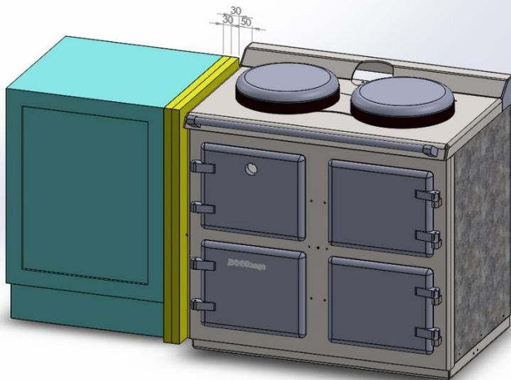
If you want to bring the cupboards closer, then you must add insulation about 75mm thick. We recommend a material called calcium silicate boards which is very effective and we can supply 100cm by 90cm boards. These are 30mm thick. You must still leave a 50mm gap to the cooker for air supply and cooling. Alternatively, a small brick stud wall can be built.
